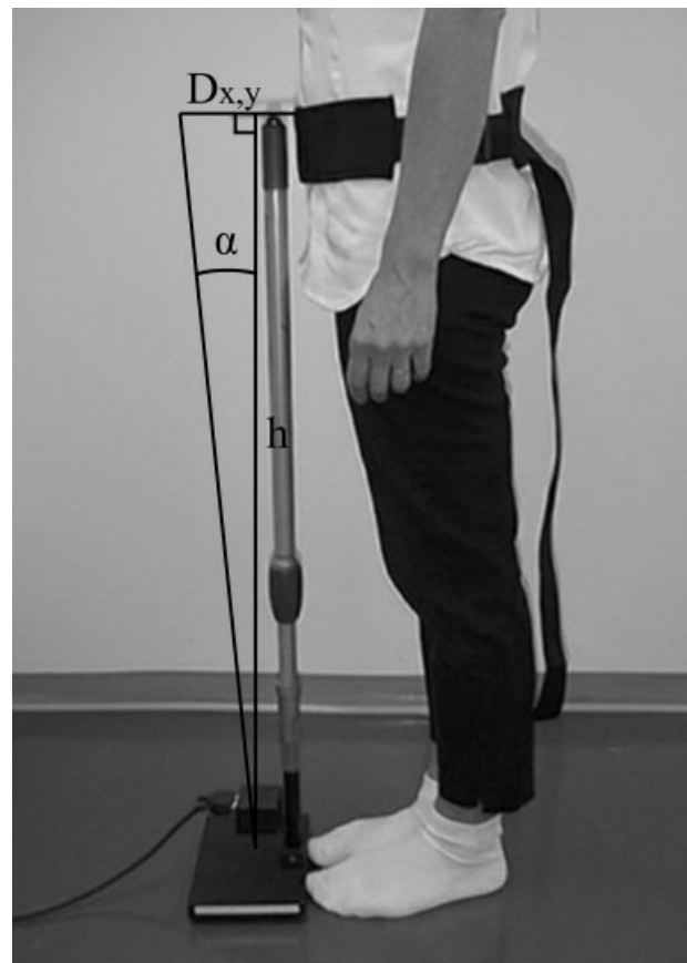
FIG. 1. The inclinometric single-link pendulum device for assessing postural sway consists of a belt fastened firmly to a subject at the level of the sacrum, an inflexible measuring rod, an inclinometric module, and a joint structure lying on the ground connected with a power unit and a computer. The movement of the measuring rod ( D_{x,y} ) is calculated separately in lateral ( x ) and antero-posterior ( y ) directions at the level of the estimated height ( h ) of the center of gravity, \alpha being the measured inclination.
